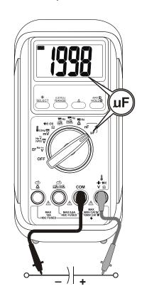
**Note:** Discharge capacitor(s) before making capacitance measurements. Large-value capacitors should be discharged through an appropriate resistance load. Using the Capacitance function in a live circuit will produce false results and may damage the meter. In many cases, the suspected component(s) must be disconnected from the circuit to obtain accurate measurement readings.
