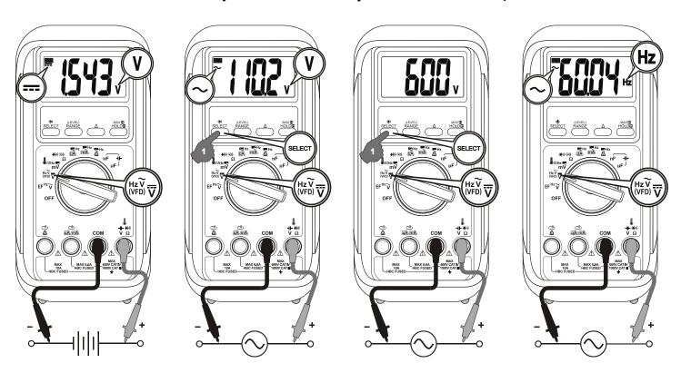
**Note: VFD-ACV** and **VFD-Hz** are equipped with a digital low-pass filter (DSP) and are capable of handling **VFD** (Variable Frequency Drives) signals for fundamental V & Hz readings. It also improves ACV and Hz reading stability when being used in most electrically noisy environments.
